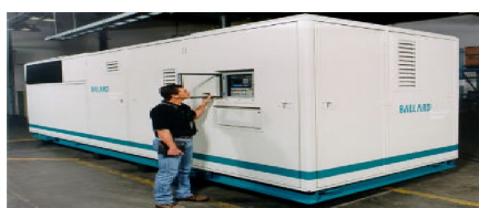
PEM plant, provides 250 kW enough to power a small building as a school or a community of up to 50 houses.
