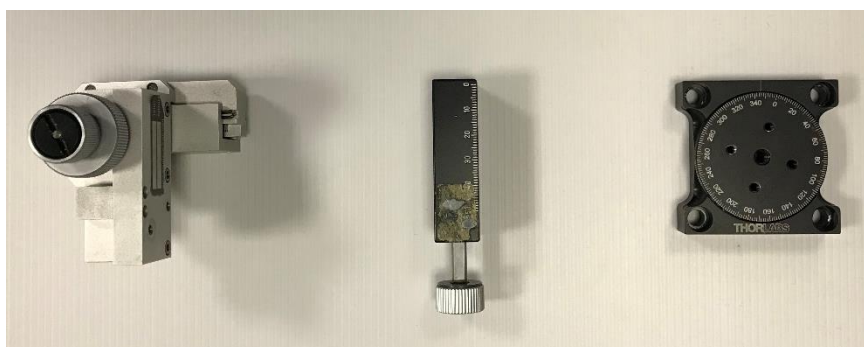
Fig 5.10: Left: commercial y- and z-positioners used. Centre: commercial x-positioner used. Right: commercial rotation angle mount used.
