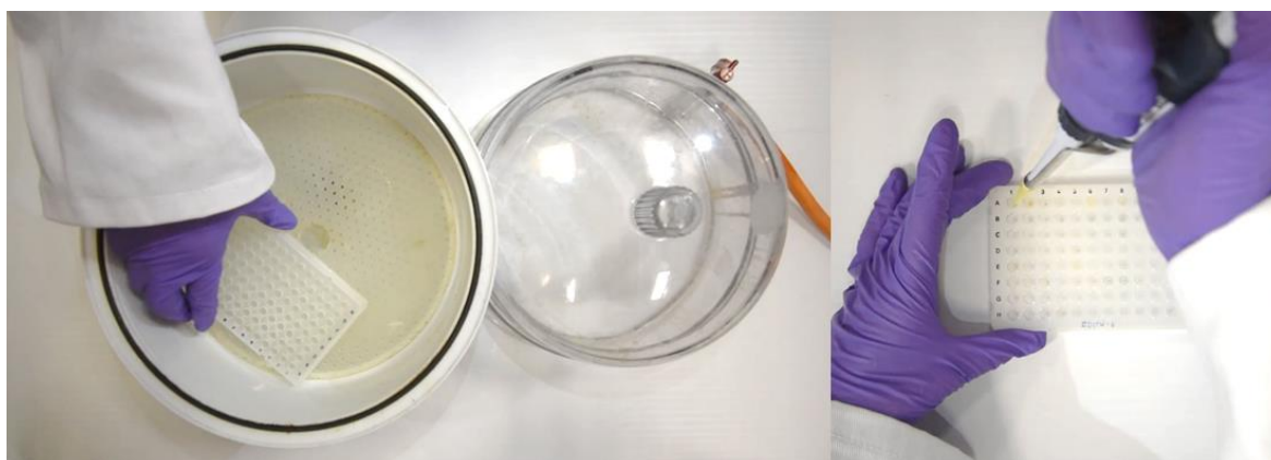
Figure 3.14: Left: Placing the 96 well plate with the samples in the desiccator. Right: Reconstituting the samples in the wells.
