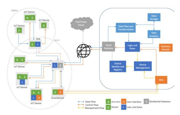
Note: Smart Home architecture example with the three viewpoints merged. Adapted from: Ghirardello, K., Maple, C., Ng, D., & Kearney, P. (2018). Cyber security of smart homes: development of a reference architecture for attack surface analysis. IoT.
