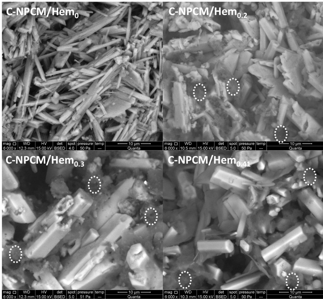
Fig. 3. SEM images of gypsums with different NPCM/Hem mass ratio.
