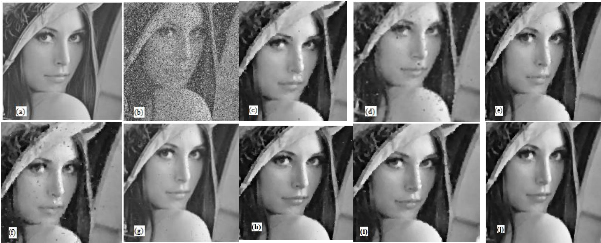
Figure 8. (a) Shows zoomed Lena image. (b) Noisy image with 40% RVIN. De-noised images using (c) DWM, (d) NWM, (e) AEPWM (f) SRM, (g) AFIDM, (h) QSAF, (i) TSA and (j) Proposed.
