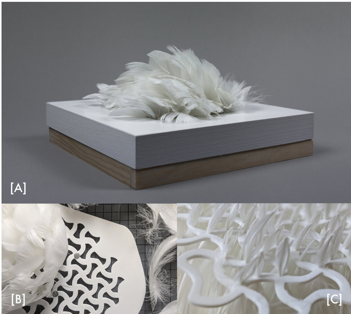
Fig. 5. (A) illustrates the material swatch of the feathered, shape-changing surface to explore the movement behavior, (B) presents the fabrication of the feathered, shape-changing textile, and (C) depicts a close-up of the feathers combined with the auxetic structure.
