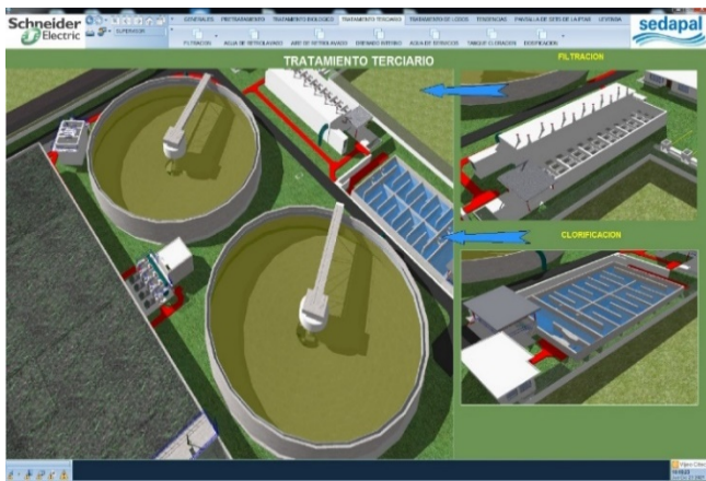
Fig. 2. Bioreactor and settling tanks.
