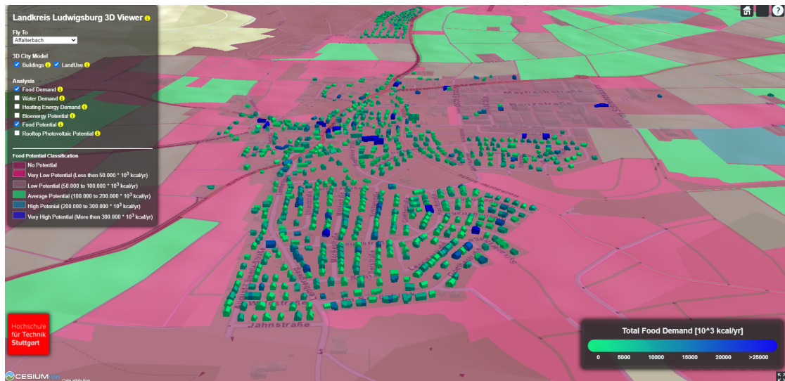
Figure 3.1: Visualization screenshot of food demand (per building) and food potential (per field polygon around settlement areas) in Affalterbach, Ludwigsburg.
