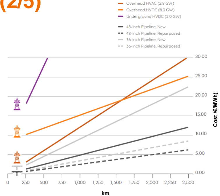
Figure 31. Cost comparison of electricity and hydrogen infrastructure assuming hydrogen as end product. Source: [47].
