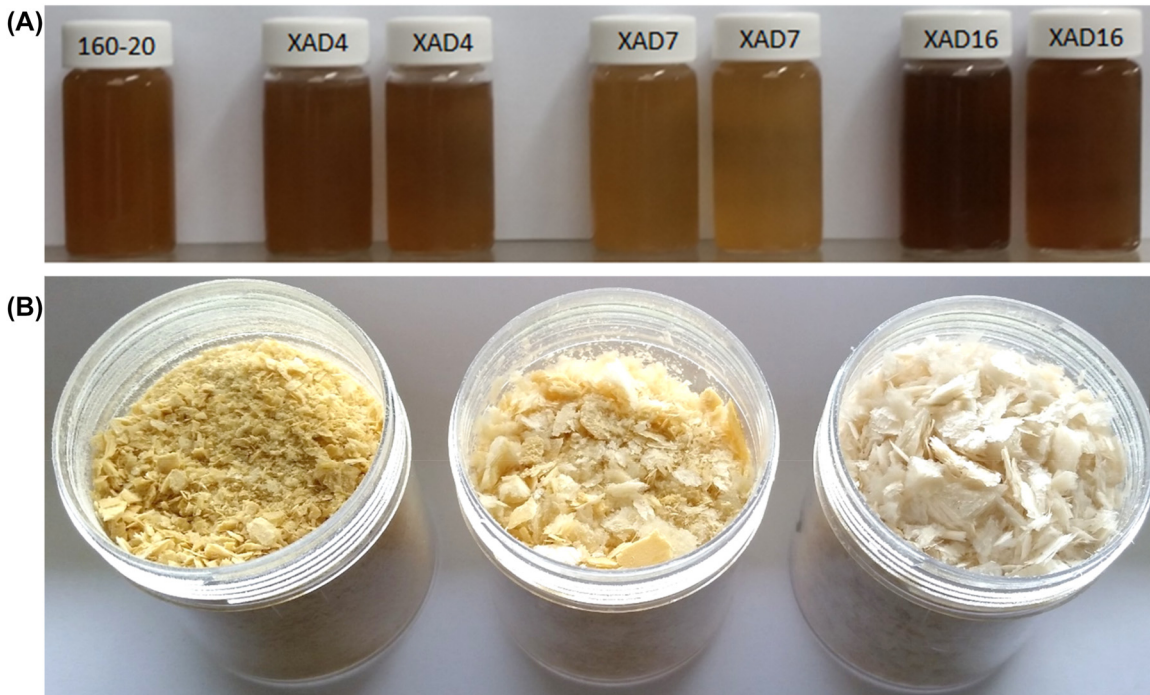
Figure 4: Unpurified and purified compression screw pressates (CSPs) before and after drying. (A) Compression screw pressate (CSP) 160/20 before (left) and after treatment (XAD samples). In each pair of XAD samples the sample on the left is from a single treatment and the sample on the right from two successive treatments with fresh resin (1 h; resin-to-liquid ratio 0.08; 24 °C). (B) Freeze-dried CSP samples: 160/20 before XAD7 treatment (left), after XAD7 treatment for 3 h at 24 °C (middle) and the high-MW fraction (retentate 2 of Table 3) isolated by ultrafiltration (right).
