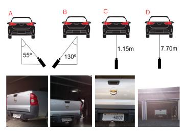
**Figure 6.** Camera positioning: (**A**) minimum angulation; (**B**) maximum angulation; (**C**) minimum distance; (**D**) maximum distance.
