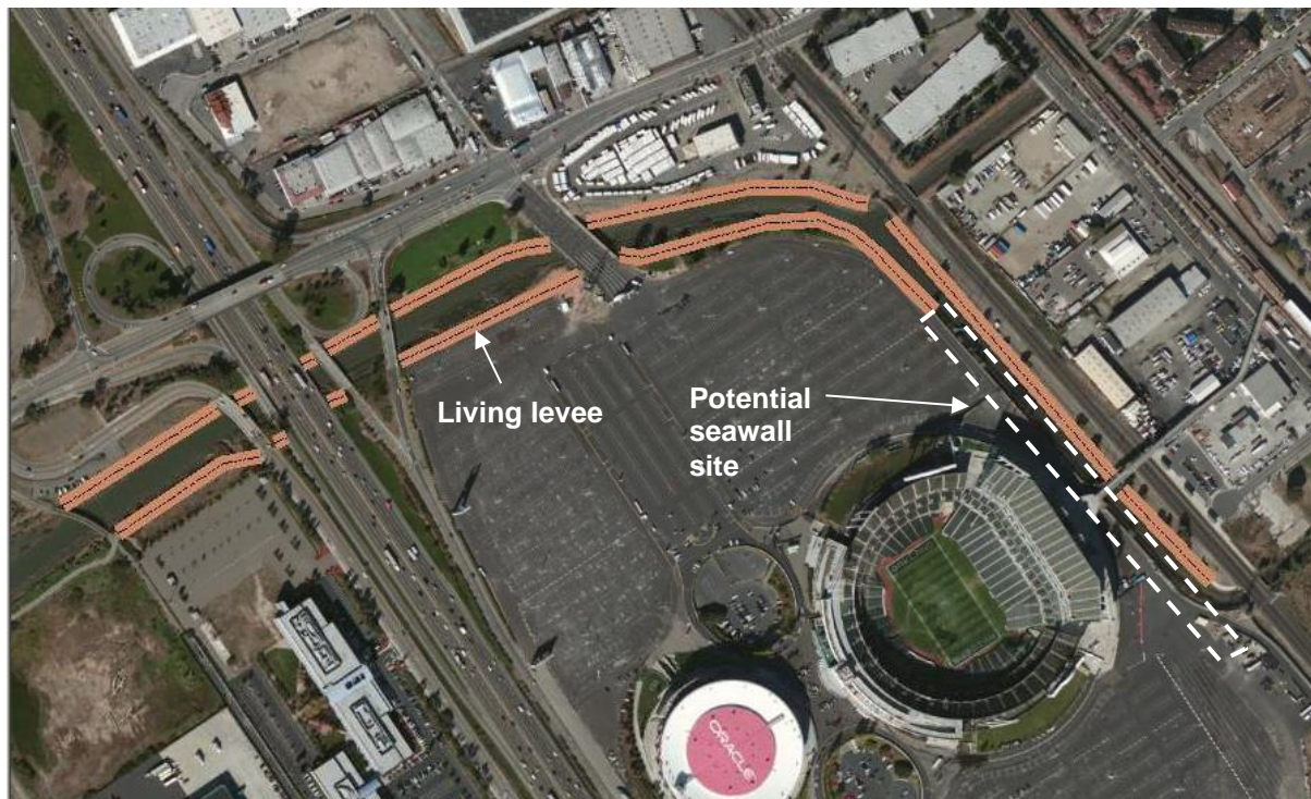
Figure 6-5: The layout and footprint of the living levee (brown) and the section where seawall might be necessary due to space limitations
