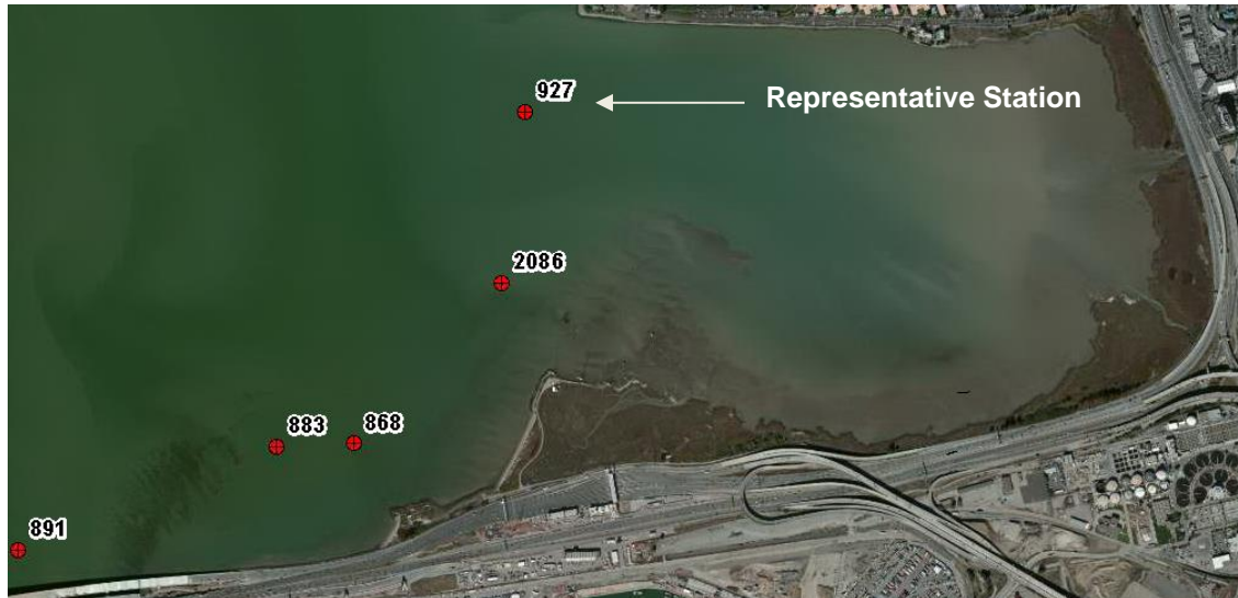
Figure 5-4: MIKE21 model output stations selected to assess both swell and seas conditions within the focus area. Station 927 was used as a representative station
