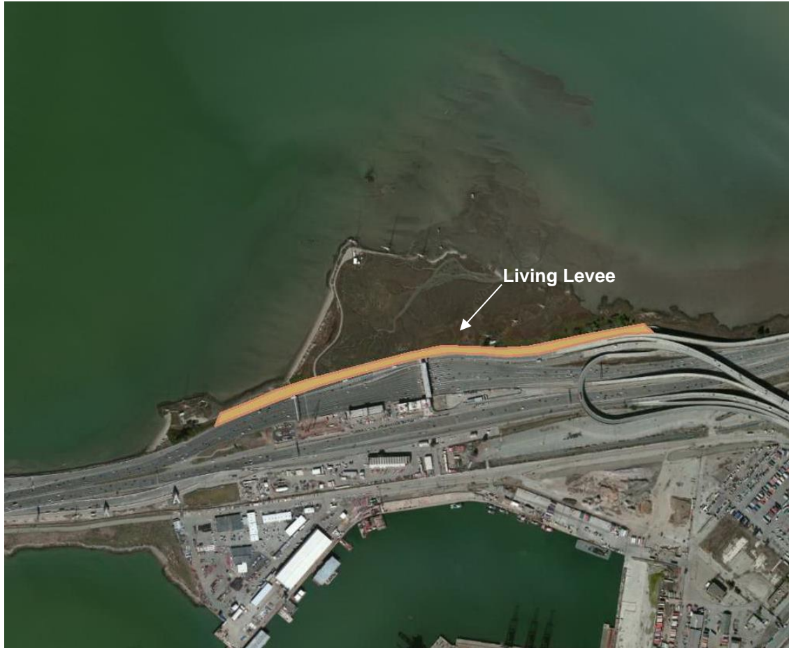
Figure 5-10: Approximate footprint of the living levee designed to protect I-80 from inundation under 36 inches of SLR. This particular placement will protect the three inundated (sites A, B, C in Figure 5-2)
