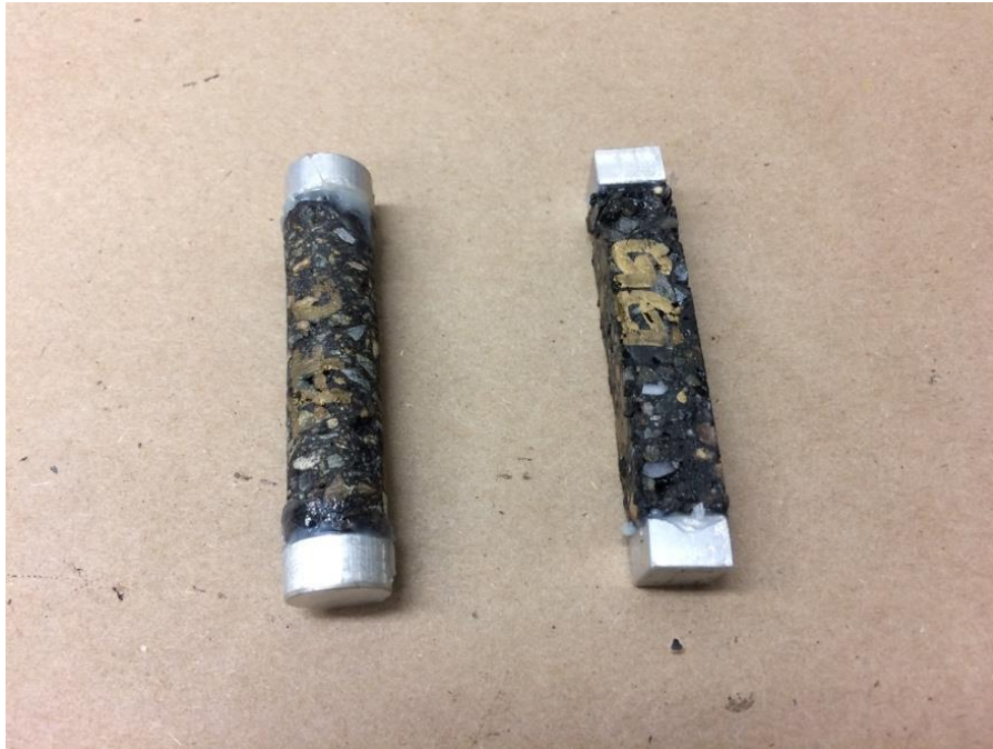
Figure 7.9 FAM specimen preparation: gluing studs (left side shows standard cylindrical FAM specimen, right show rectangular FAM specimen).
