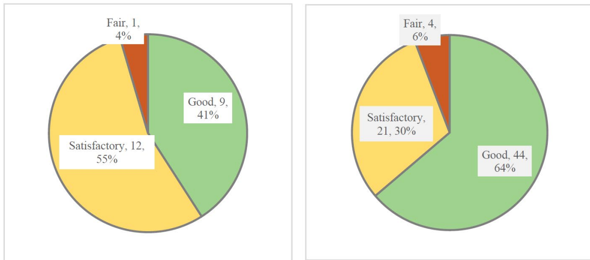
Figure 7-3: Summary of condition state distribution for all Geotechnical Assets on NHS routes in the Northwest District (left) and Northeast District (right).
