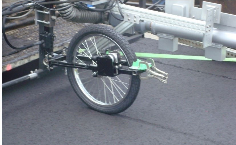
Figure 10. Demo No. 1 - ARTS Distance Measurement Instrument (DMI).
