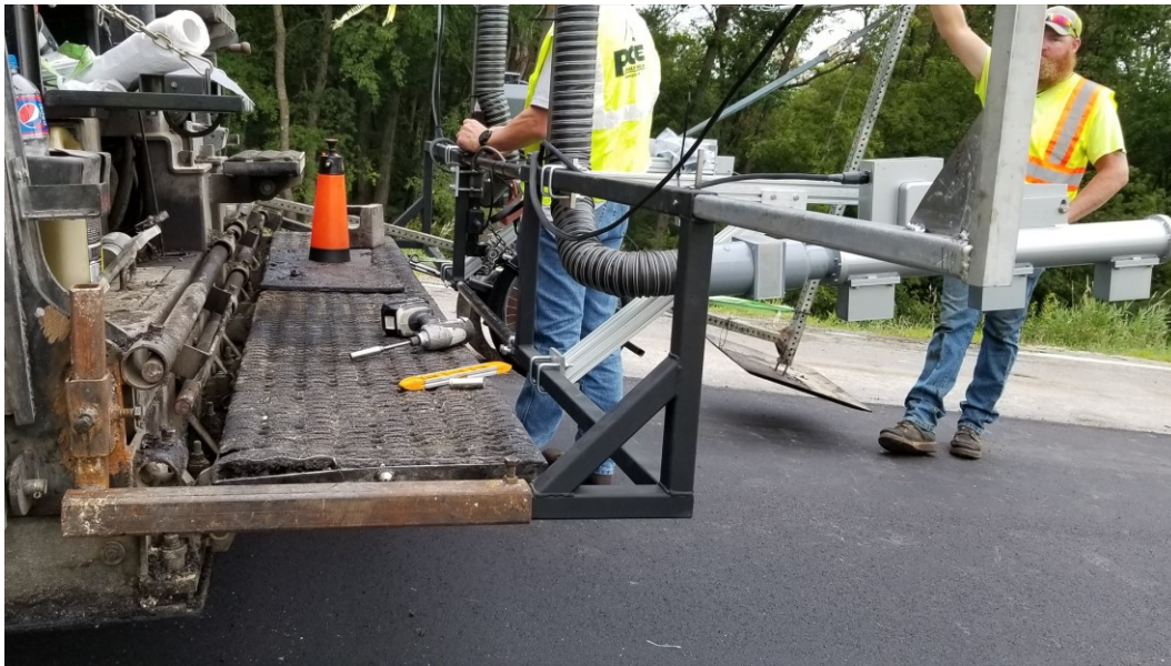
Figure 4. ARTS sensor assembly by Vendor A connected to the receiving bracket on the left side of a paver screed.
