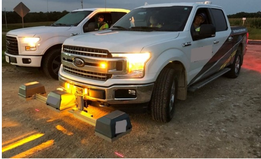
Figure 14. Demo No. 1 - Vendor A's highspeed inertial profiler.
