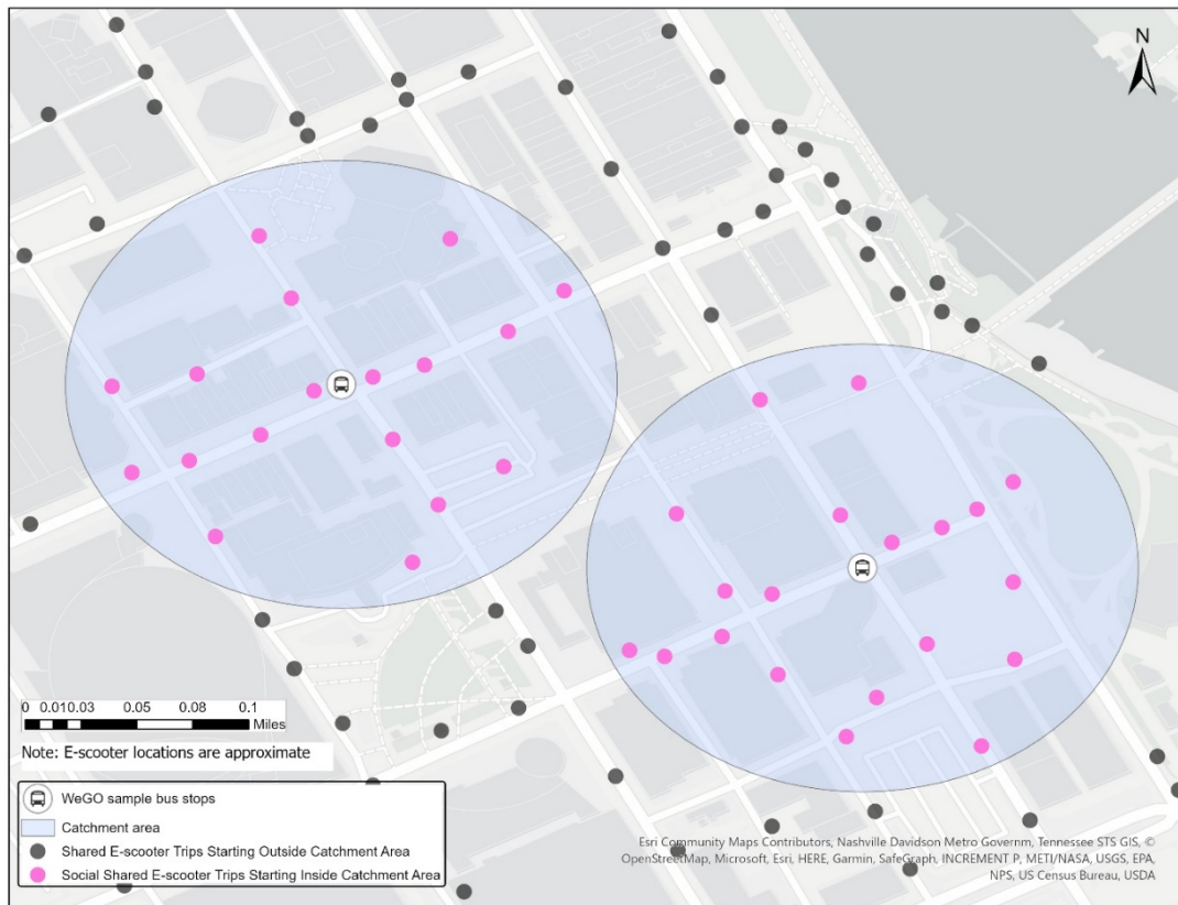
Figure 8: Example of shared e-scooter trips assignment method to bus stops
