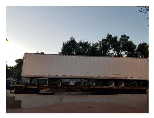
Figure 17: A "Trailer-on-Flatcar," or TOFC, Going through the Davis, CA Station
