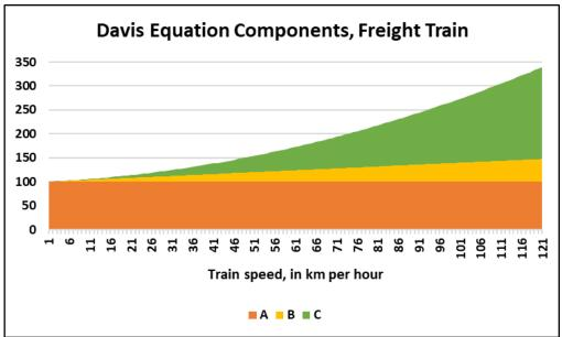
Figure 9: Resistance Forces versus Train Speed (Passenger example based on Capitol Corridor; freight example based on KC-to-Wellington freight route. Both routes are described in further detail, below.)
