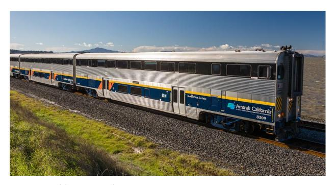
Figure 21 "California Cars," the Railcars Typically Used along the Capitol Corridor Route Photo courtesy of Rob Edgcumbe, and Caltrans (with permission granted)
