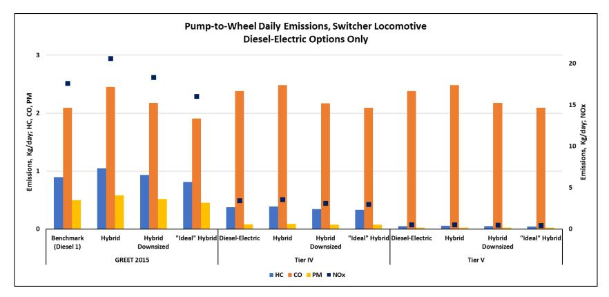
Figure 53: Pump-to-Wheel Daily Emissions, Switcher Locomotive, Diesel-Electric Options Only HC, CO, and PM are indicated by columns, while NOx levels are indicated via a square notation.
