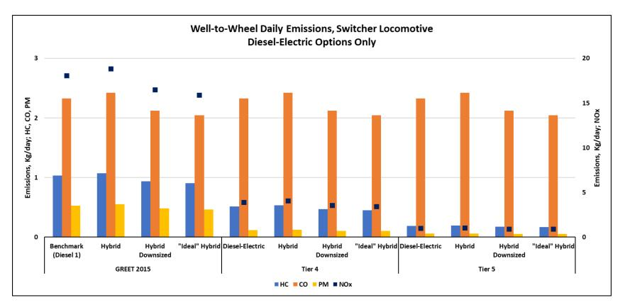
Figure 54: Well-to-Wheel Daily Emissions, Switcher Locomotive, Diesel-Electric Options Only
