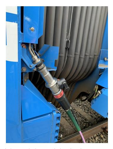
Figure 58: Refueling a Multiple Unit Vehicle with Hydrogen Photo courtesy of Dr. Andreas Hoffrichter
