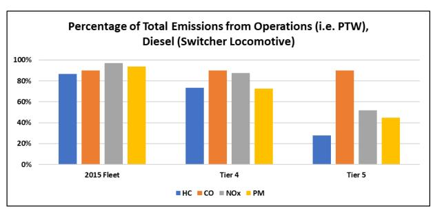
Figure 52: Percentage of Total Emissions from Operations (PTW), Diesel, Switcher Locomotive
