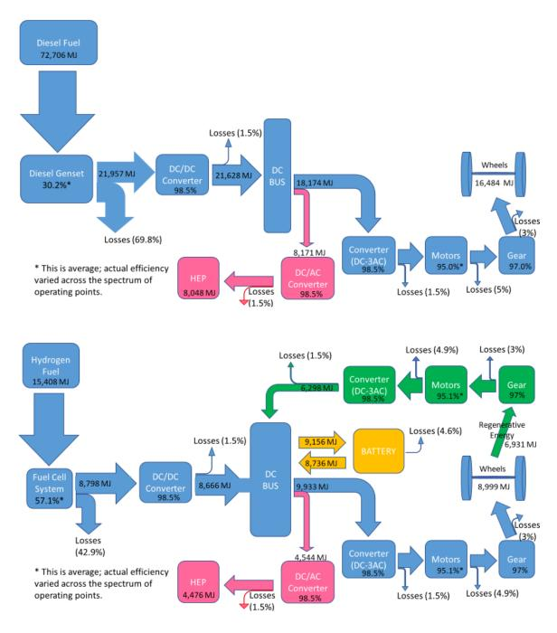
Figure 27: Diagrams of the Flow of Energy for Two of the Simulated Powertrains
