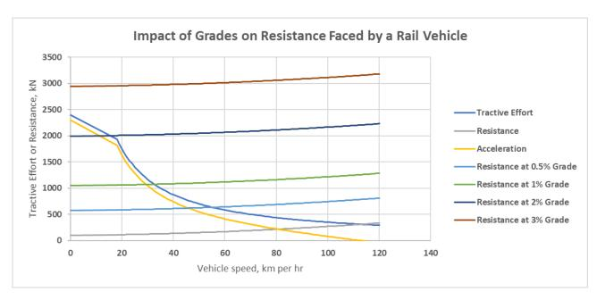
Figure 18: Impact of Grades on Resistance Faced by a Rail Vehicle
