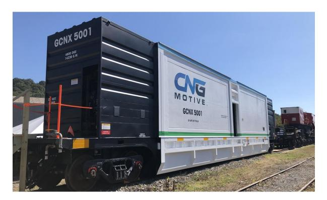
Figure 4: A CNG Tender Recently Developed by CNGmotive
