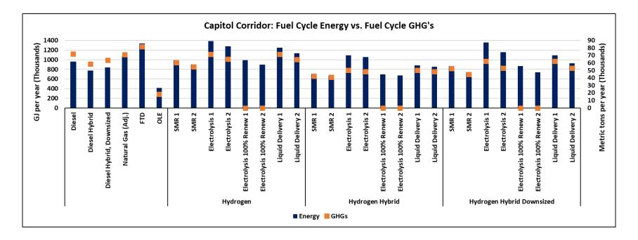
Figure 38: Fuel Cycle Energy vs. Fuel Cycle GHG's.
