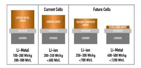
Figure 8: Potential Future Improvements, Energy Density, Lithium Ion Cells.
