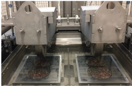
Figure 3.2 INDOT HWTT set up.
