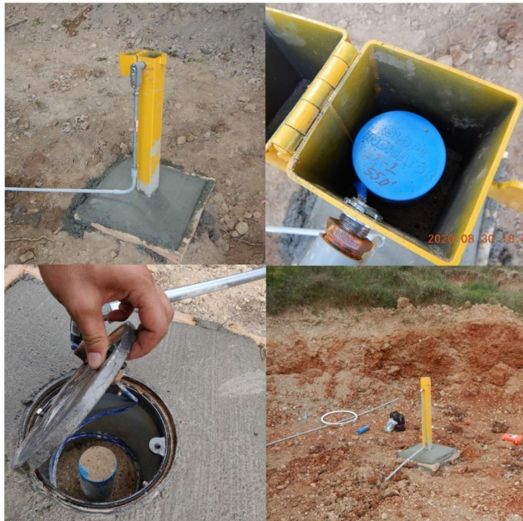
Figure 16: SI Monuments at Branson Landslide. Clockwise from top left: LT-1 above-ground monument, LT-1 open showing inclinometer pipe, LT-2 above-ground monument, and LT-3 flush mount.
