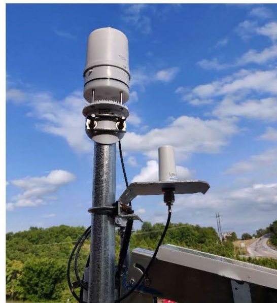
Figure 18: Pair of photos showing weather station as installed at base station (left) and a close up of the weather station and sensor (right).
