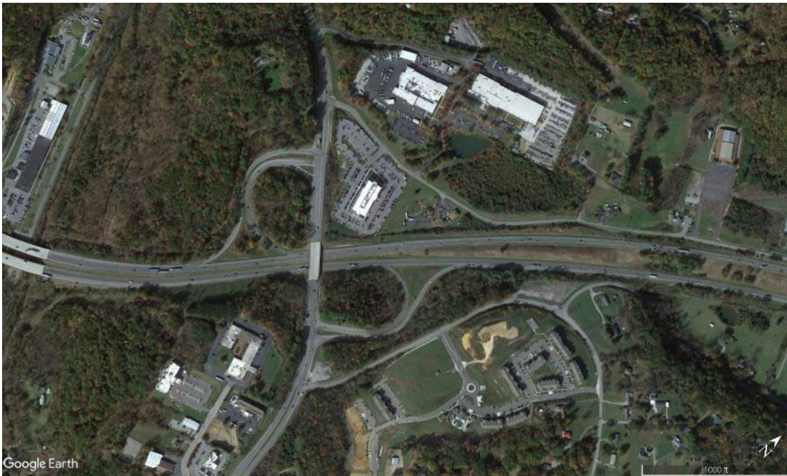
Figure 17. Photo. Aerial image of a parclo B2 interchange. (10)
