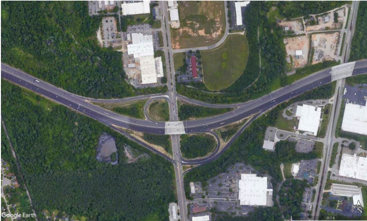
Figure 18. Photo. Aerial image of a parclo B4 interchange. (10)
