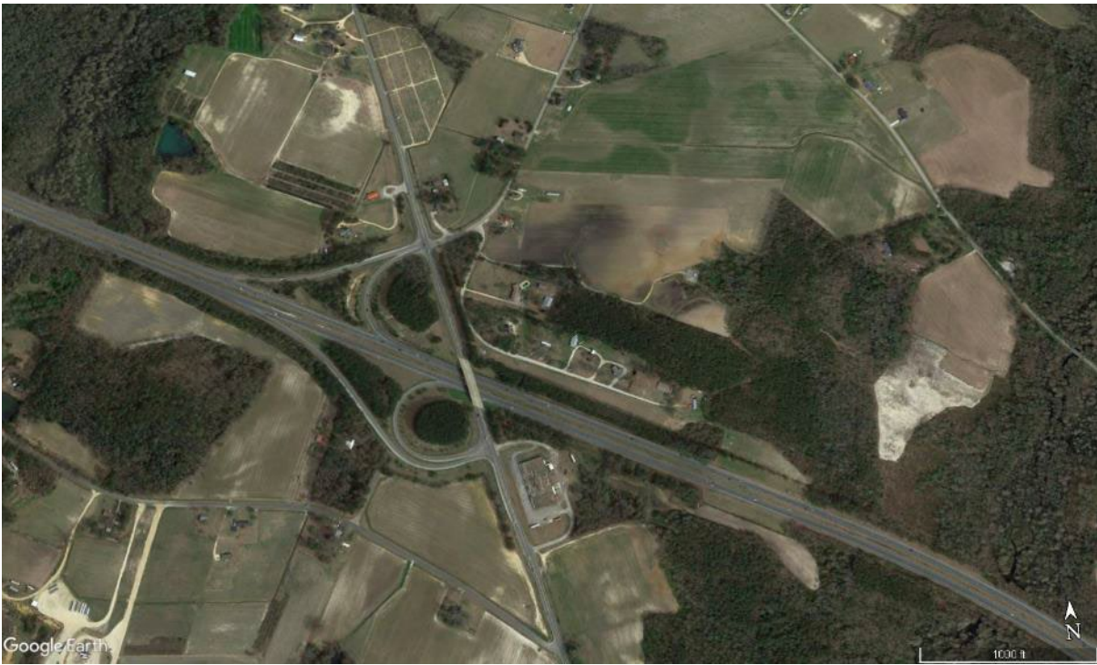
Figure 19. Photo. Aerial image of a parclo AB2 interchange. (10)
