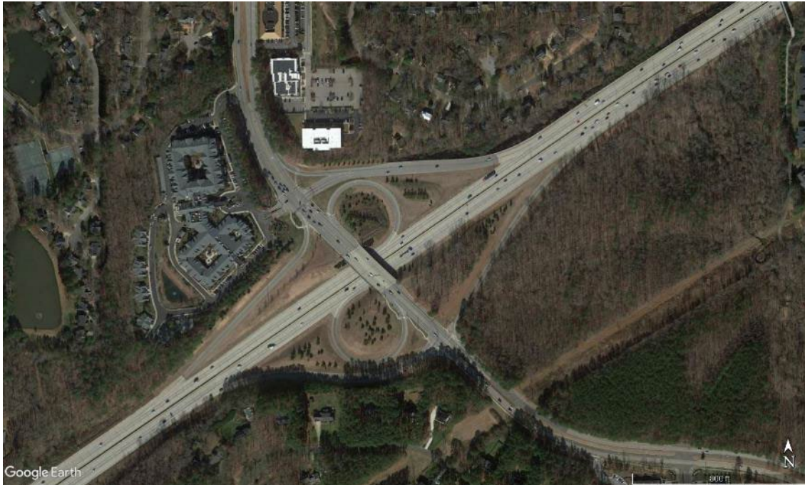
Figure 16. Photo. Aerial image of a parclo A4 interchange. (10)
