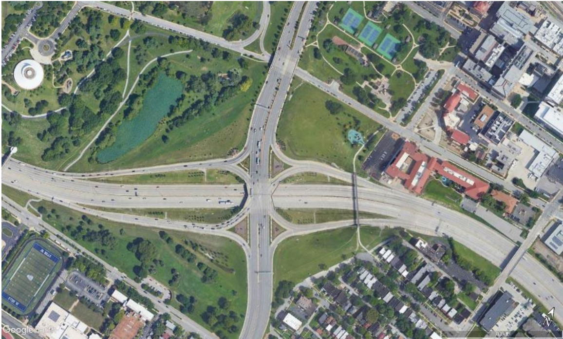
Figure 14. Photo. Aerial image of an SPDI. (10)
