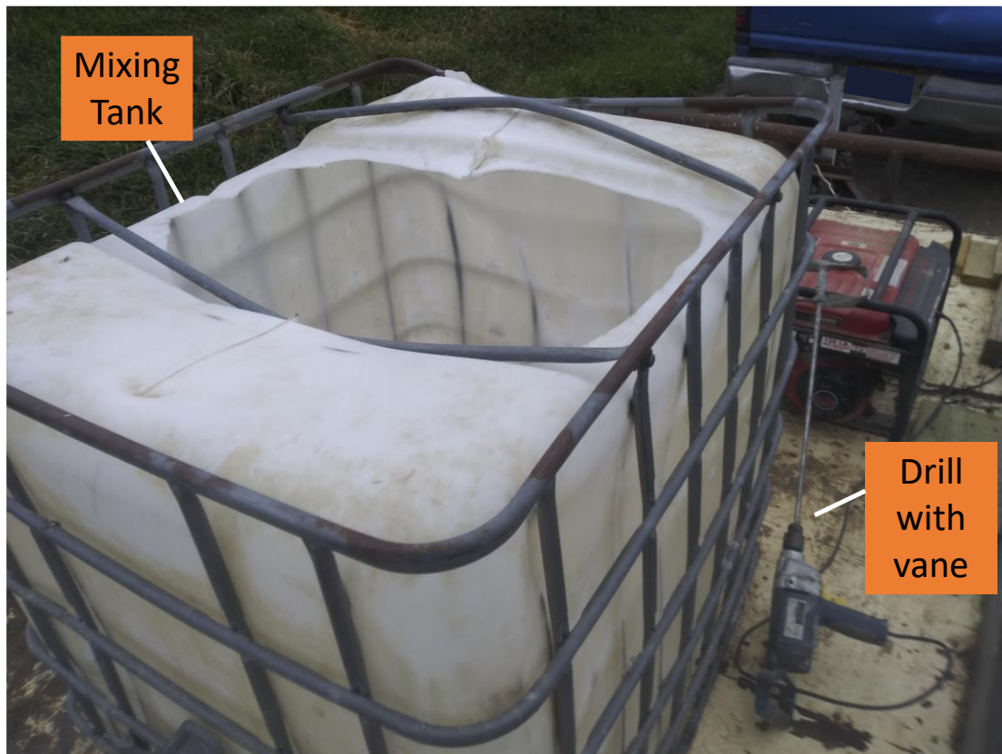
Figure 4-3 Mixing tank and ½ hp drill with a mixing vane.
