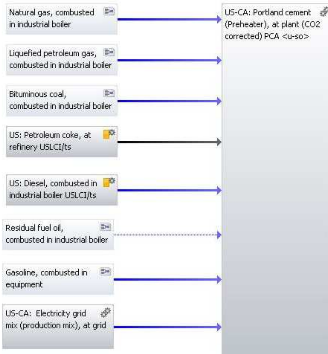
Figure 3.20: The model for cement production (preheater method + CA electricity mix.)
