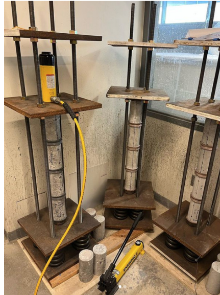
Figure 2. Creep frame with specimens under load
