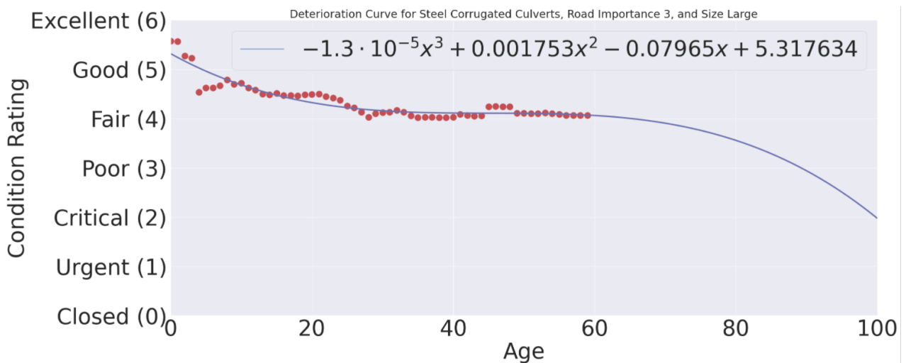
Figure 26-Deterioration curve for steel corrugated culverts with Random Forest, RI = 3
