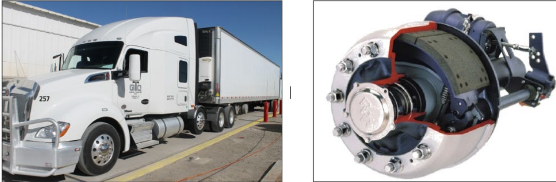
Figure B-1. 2010 Freightliner Cascadia with sleeper in a 3-axle all drum configuration + 53' dry van trailer with a 2-axle all drum configuration + Drum Brake.
