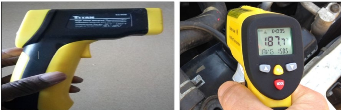
Figure B-3. Hand-held sensors used to take brake temperatures.
