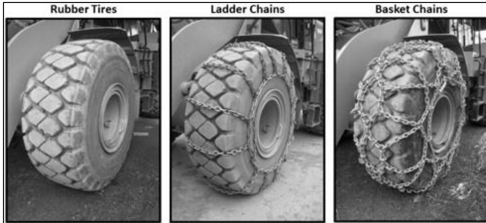
Figure 65. Tire chain configuration tested in Blood et al. (56)
