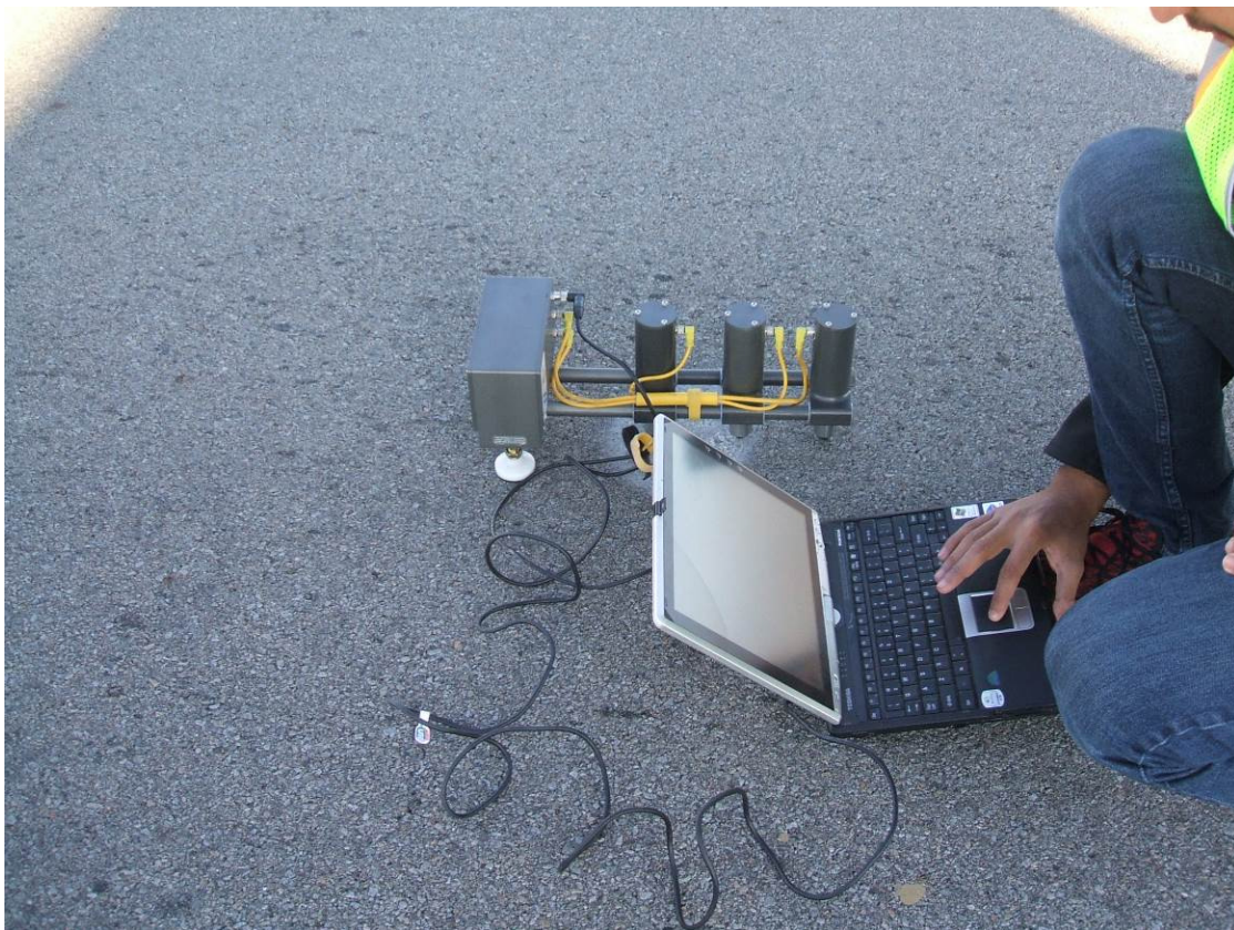
Figure 3. PSPA in operation.
