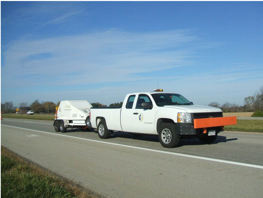
Figure 4. FWD trailer on site.
