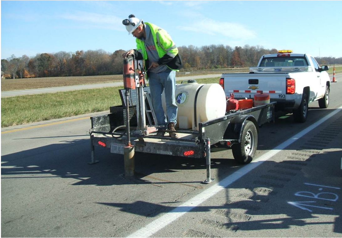
Figure 6. Drilling a 6 in (152 mm) core specimen.
