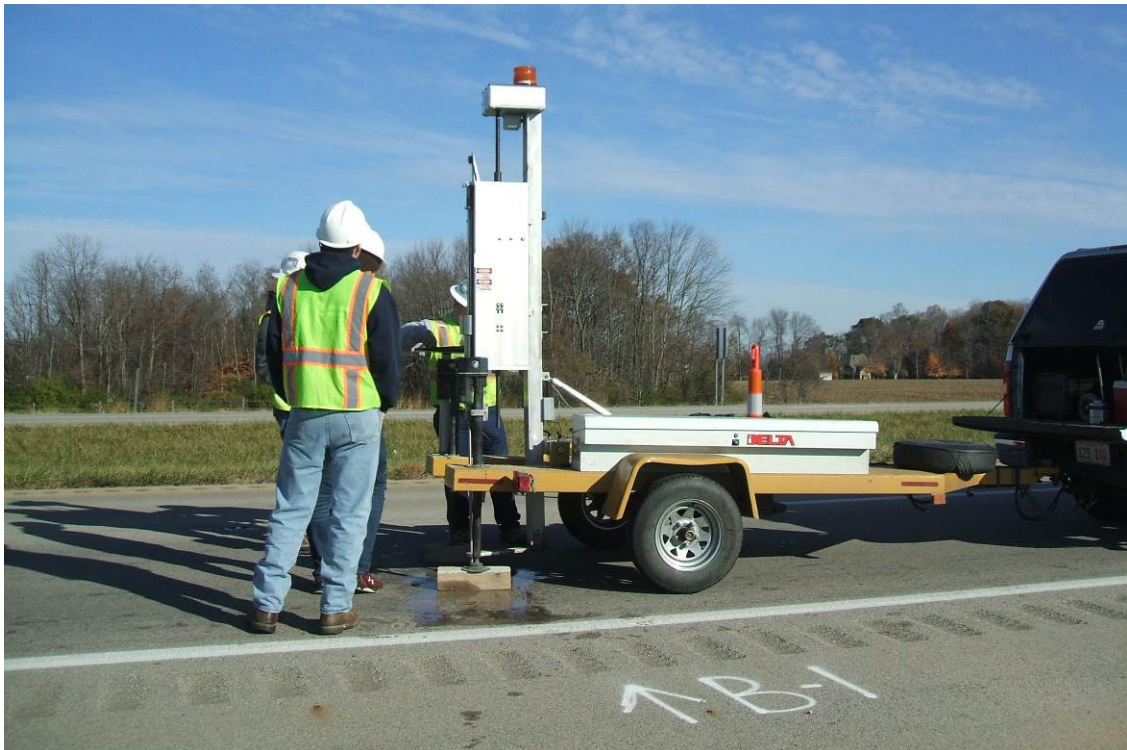
Figure 7. Dynamic Cone Penetrometer (DCP) testing.
