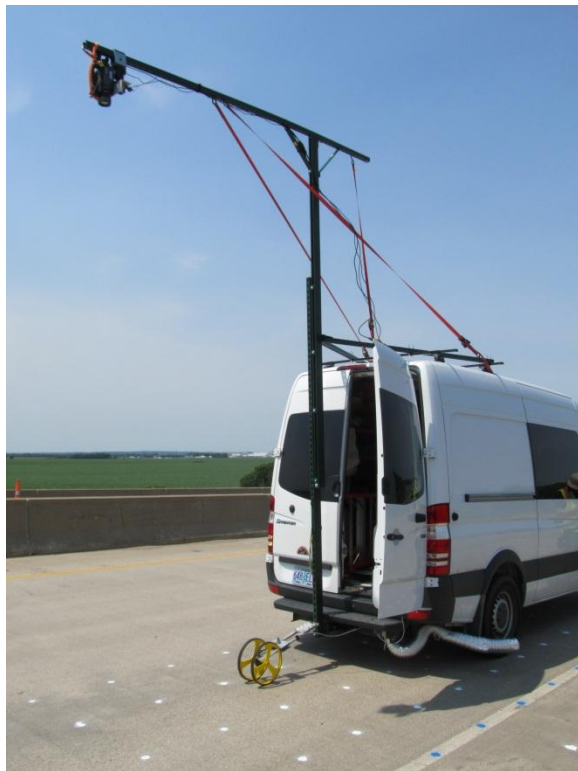
Figure 3.2. Truck equipped with infrared camera, optical camera, and encoder wheel for measuring distance travelled.
