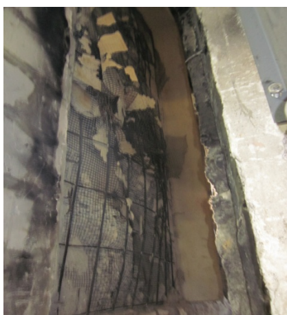
Figure 12. The 1 st test - fire exposed side, after fire test
