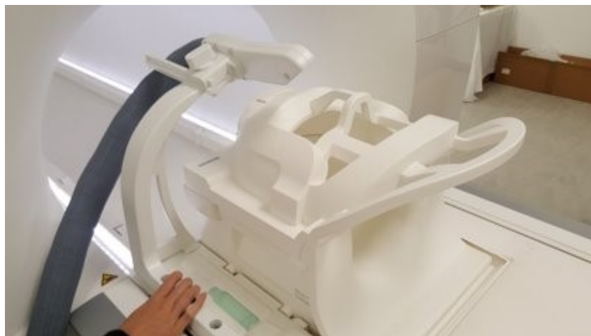
Figure 1.2.5: TCL camera attached to a mock Siemens scanner (ZT) positioned above a 64 channel head coil. Image courtesy of Dr Daniel Gallichan, (CUBRIC) Cardiff University.
