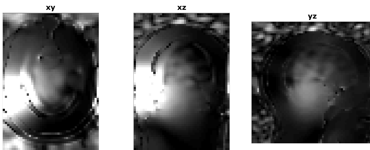
Figure 3.2.1: B_1 field maps of one channel calculated for one dataset. Maps were calculated for each channel of all the five datasets using the correspondent ACS lines acquired prior to the scan.
