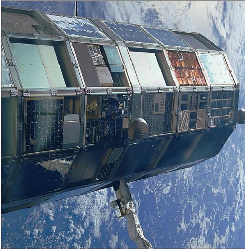
Figure 1.5. The Long Duration Exposure Facility in orbit. The various experiment trays can be seen as the individual squares on every side of the detector. The pointing of the spacecraft was maintained thus the 12 sided spacecraft allowed for experiments to be on the ram or wake facing side during the whole mission (ESA, 2009).
