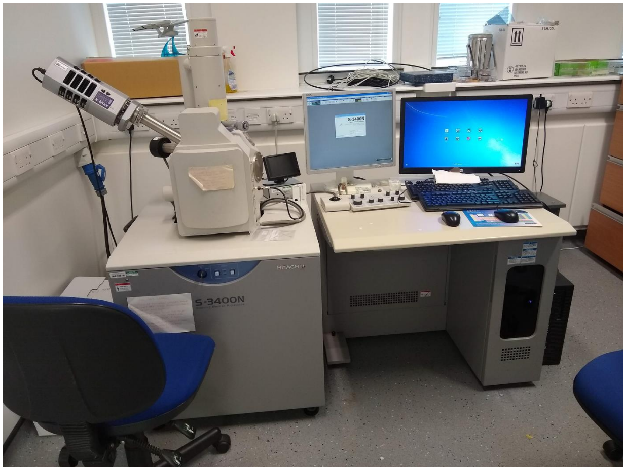
Figure 2.8. Image of the Hitachi 3400N SEM with an Oxford Instruments 80 mm 2 X-max Energy Dispersive X-ray Spectrometer at the University of Kent.
