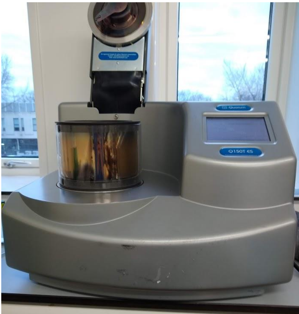
Figure 2.1. Image of the Quorum Technologies Q150T ES sputter coater with the lid of the target chamber opened.
