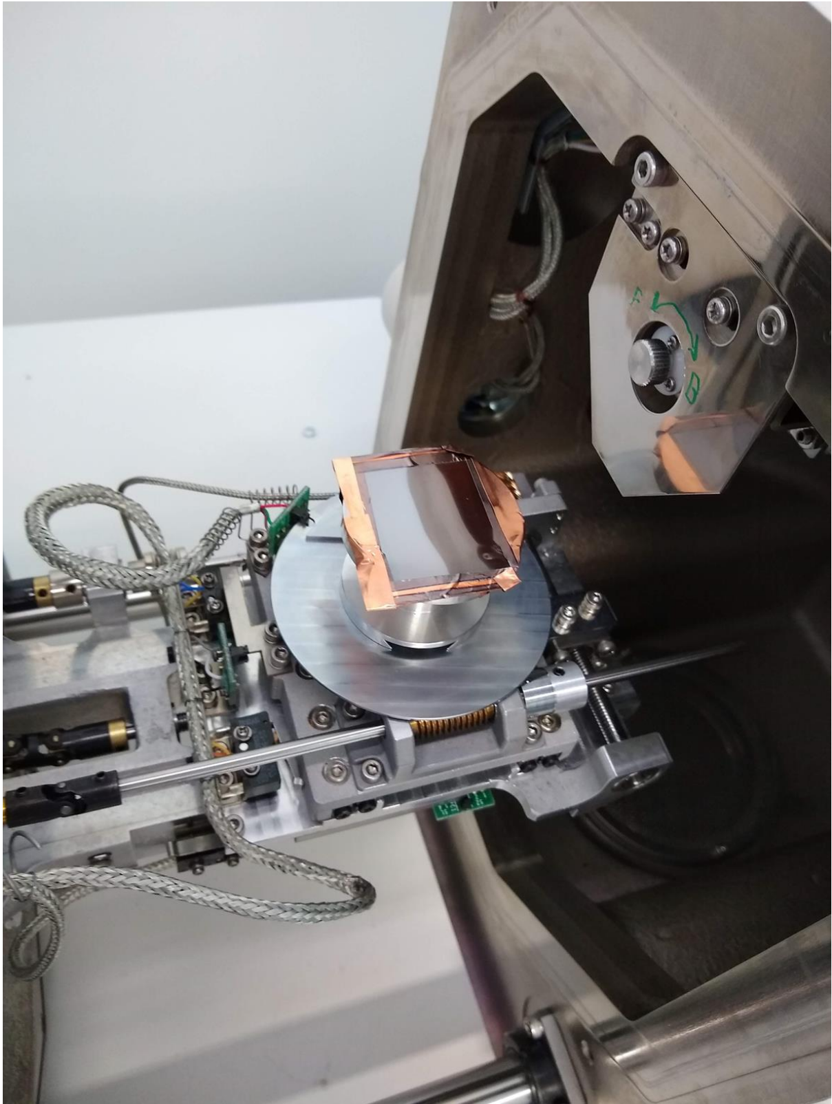
Figure 2.10. Sample mounted for SEM analysis using copper tape to hold the sample flat on an SEM stub.
