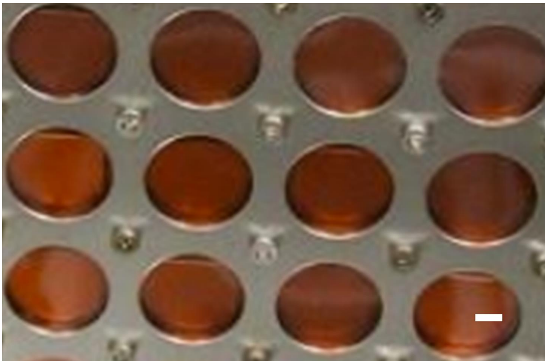
Figure 2.7. Section of the ATOX facility sample holder showing a circular region of each sample for exposure to atomic oxygen. Scalebar represents 0.5 cm.
