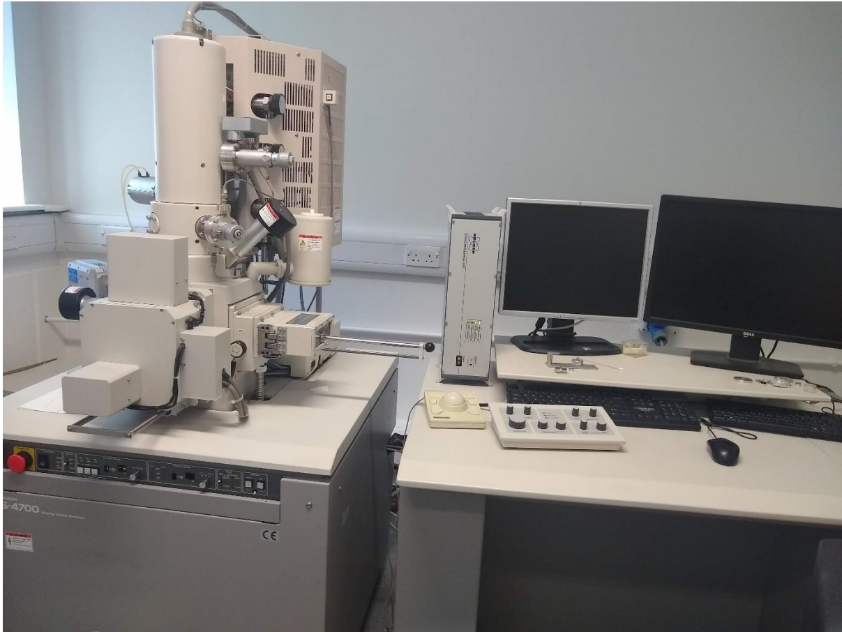
Figure 2.9. Image of the Hitachi 4700 cold field emission SEM with a Bruker X-flash Energy Dispersive X-ray Spectrometer at the University of Kent.
