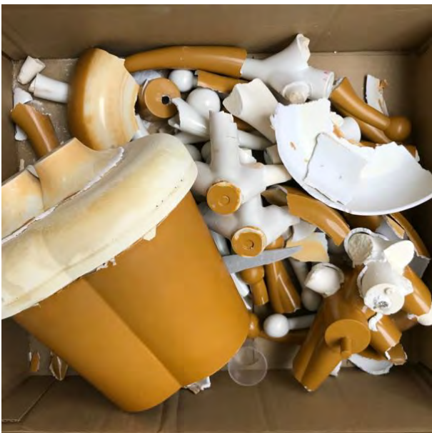
fig. 4.29 Broken plaster pattern after de-moulding
