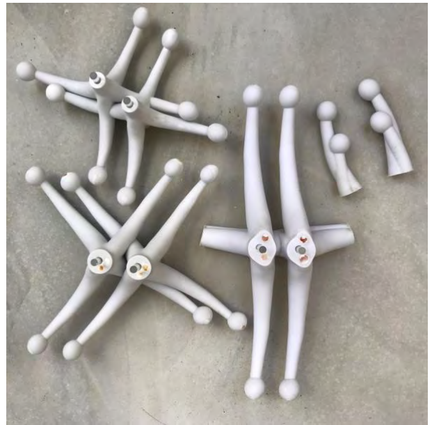
fig. 4.20 Hollow 3D prints with plaster reinforcement
