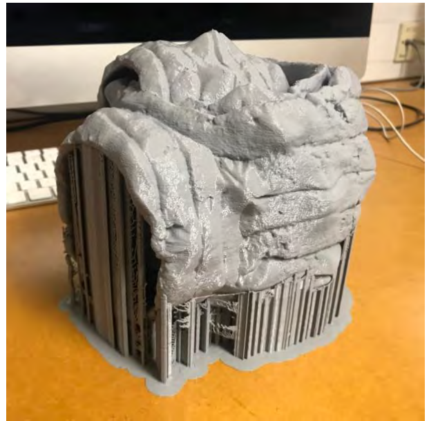
fig. 5.26 Final PLA 3D print with undercut supports
