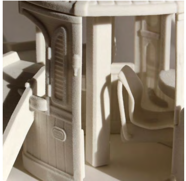
fig. 2.14 3D print of model in plaster (detail)
