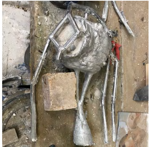
fig. 4.34 Removing runners and risers
