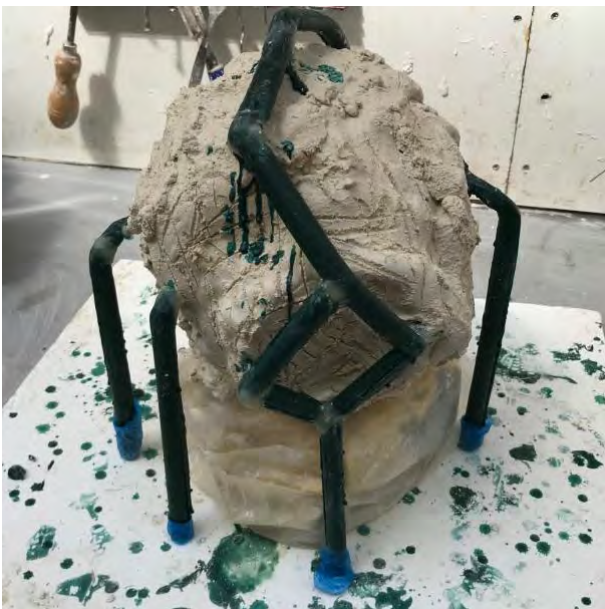
fig. 4.29 Runners, risers and airers with base shell
