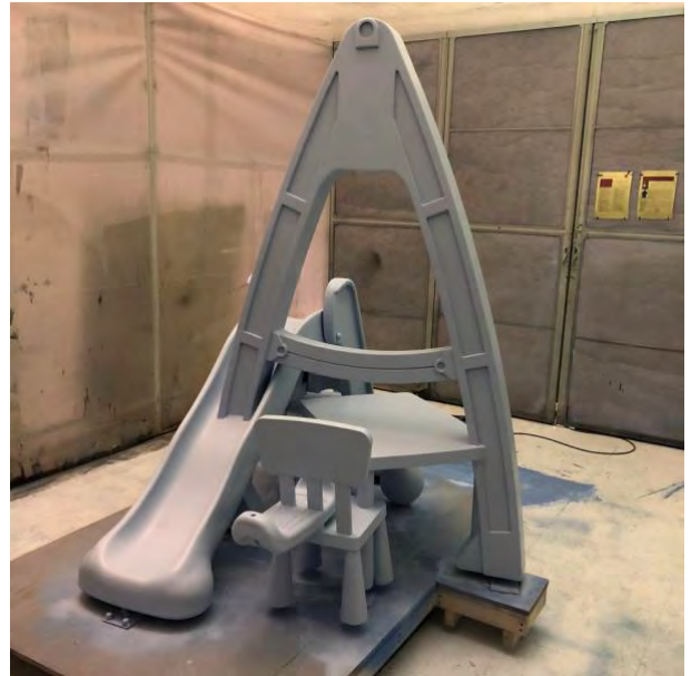
fig. 2.32 Another layer of filler-primer in the spray-booth
