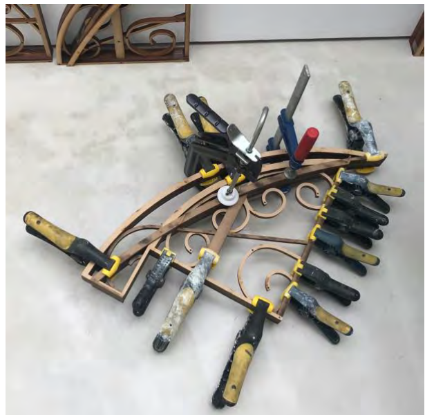
fig. 3.30 Clamping laminated sections
