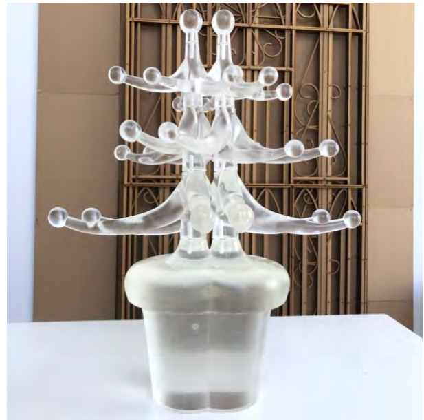
fig. 4.32 First resin cast with dowelled joints
