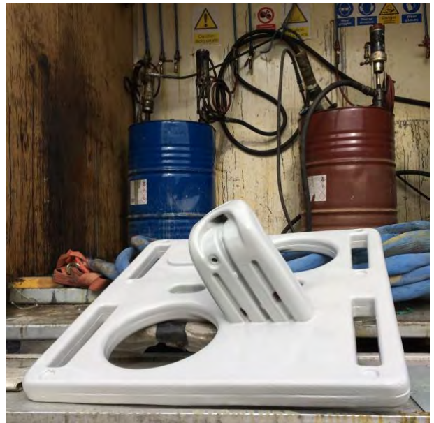
fig. 2.22 Polyurea coated prototype
