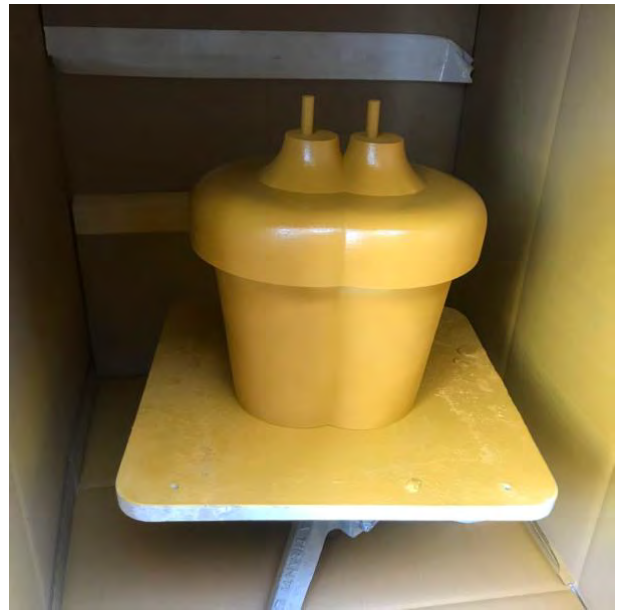
fig. 4.26 Repaired and smoothed in 'spray booth'
