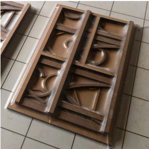
fig. 3.17 Using the bag-press to glue the layers
