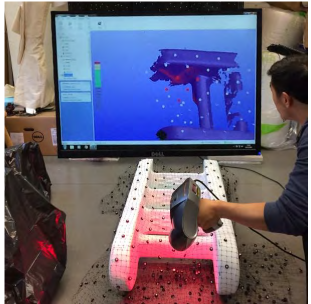
fig. 2.4 3D scanning slide ladder component at RCA
