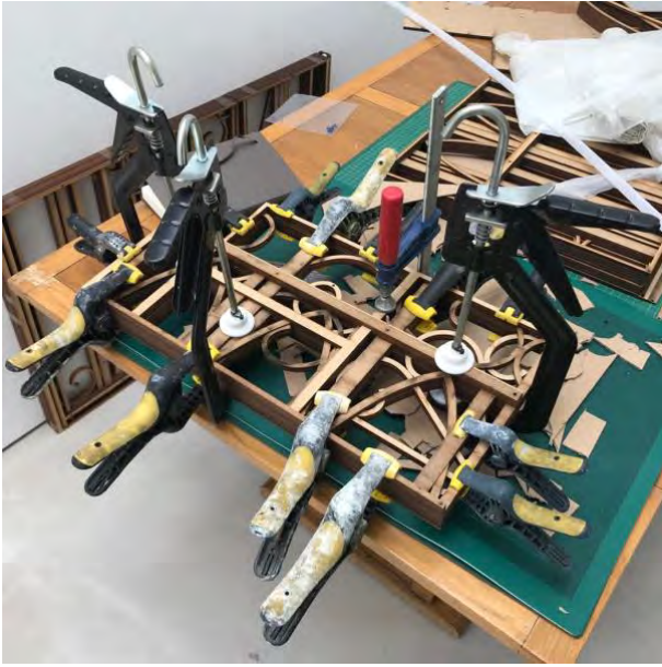
fig. 3.31 Clamping laminated sections
