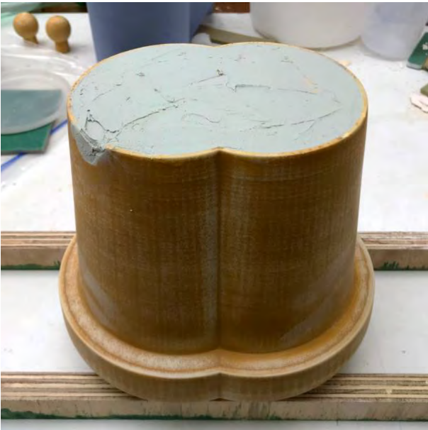
fig. 4.21 Filling the hollow 3D print with plaster
