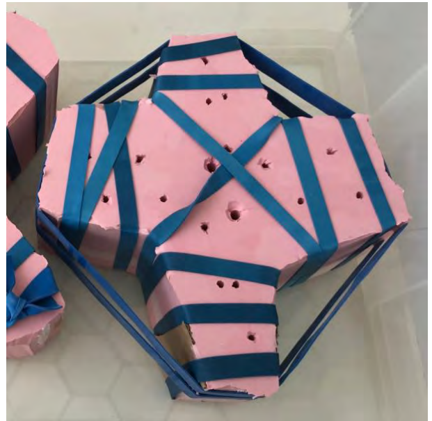
fig. 4.28 Rubber mould ready for pouring.
