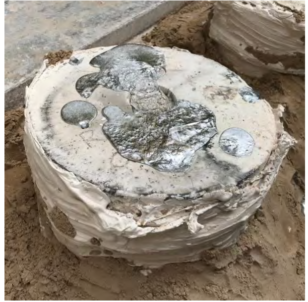
fig. 4.32 Aluminium bubbling in the mould
