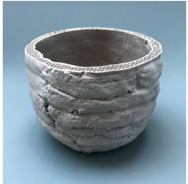
fig. 5.10 Scale 1:2 3D print (incomplete PLA/stone)
