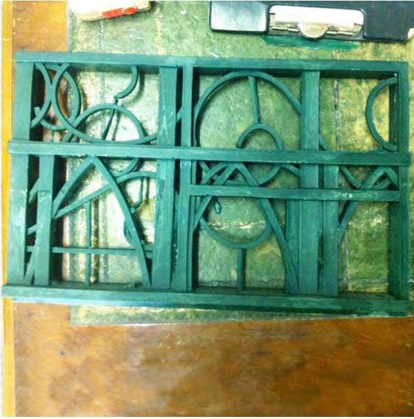
fig. 3.19 Examining a wax pattern for distortion
