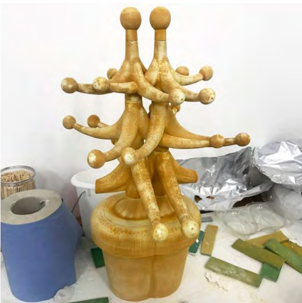
fig. 4.23 Smoothing back the textured surface
