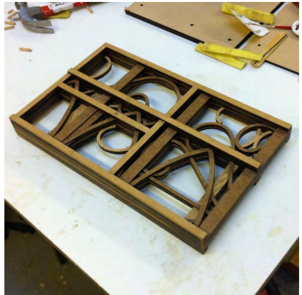
fig. 3.18 MDF pattern ready for filling and painting
