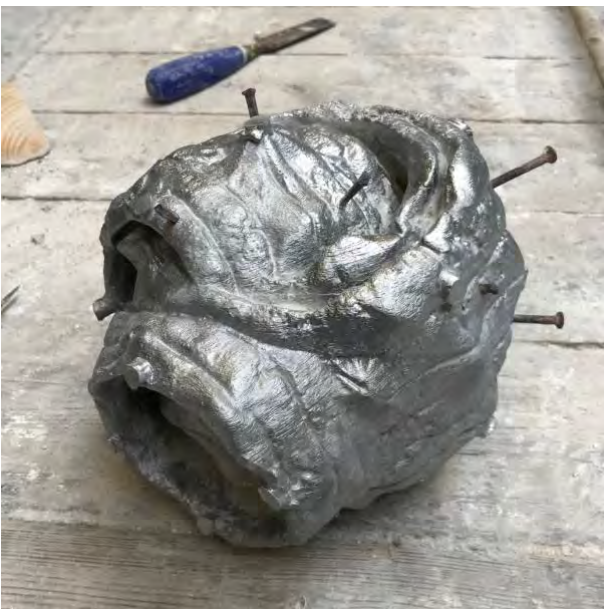
fig. 5.35 Aluminium cast with core pins still in place
