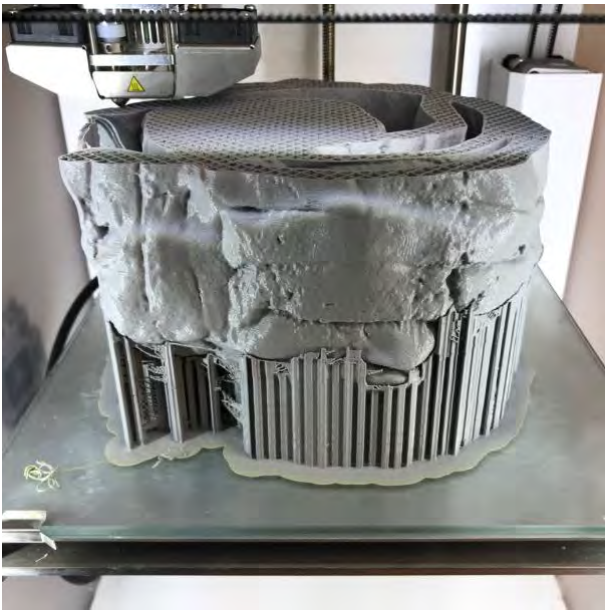
fig. 5.25 3D printing the final PLA pattern
