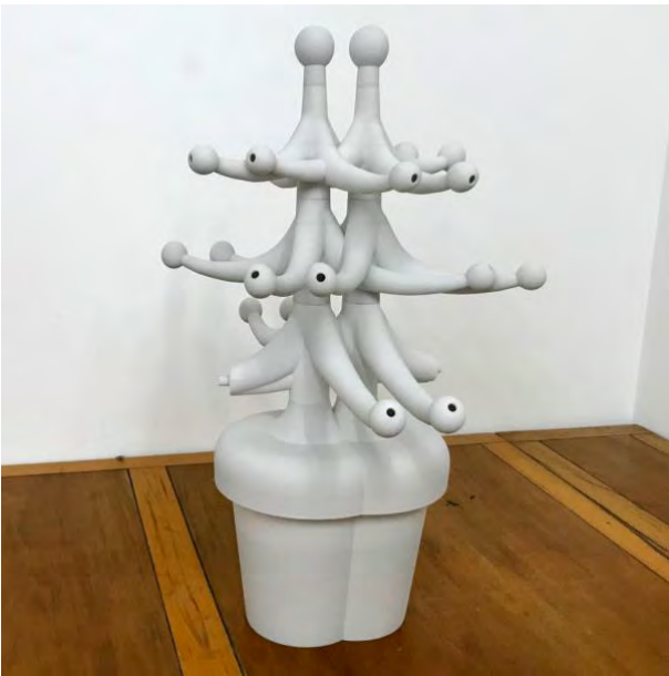
fig. 4.19 50cm hollow 3D print parts (dry assembly)
