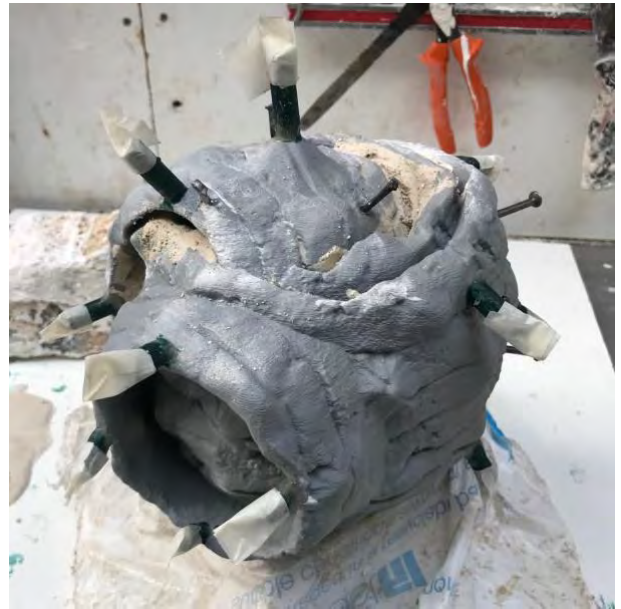
fig. 4.28 Placing runners & risers and filling cavities
