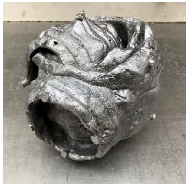
fig. 5.36 Clean aluminium cast with core pins removed
