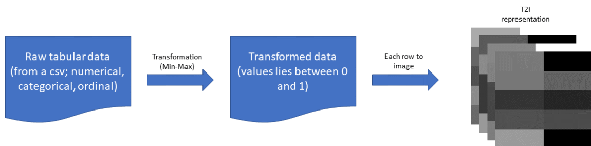
Fig. 7.1 Block diagram of T2I conversion.
