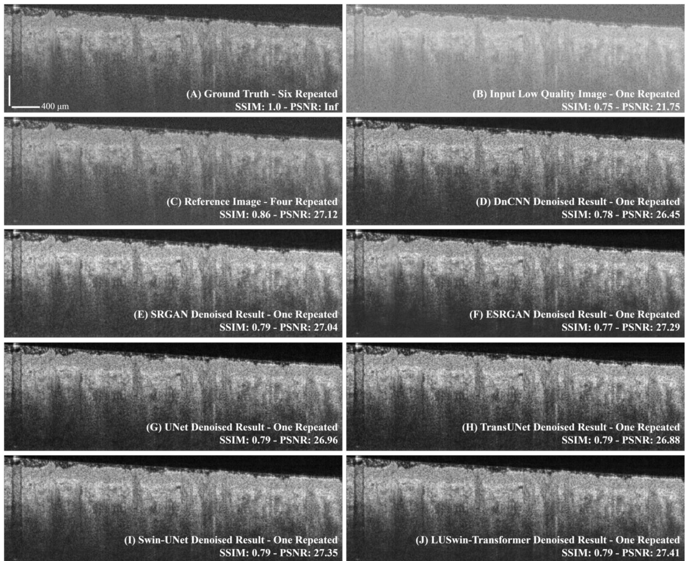
Figure A1. The visual comparison between the different methods. The image is selected from participant #011, representing the neural network performance on the face. (A) High-quality ground-truth image with six-repeated scans. (B) Low-quality input image with one-repeated scan. (C) High-quality reference image with four-repeated scans. (D–J) are neural networks denoised results from (D) DnCNN, (E) SRGAN, (F) ESRGAN, (G) UNet, (H) TransUNet, (I) Swin-UNet, and (J) LUSwin transformer. The white label is scale bar with 400 μm.
