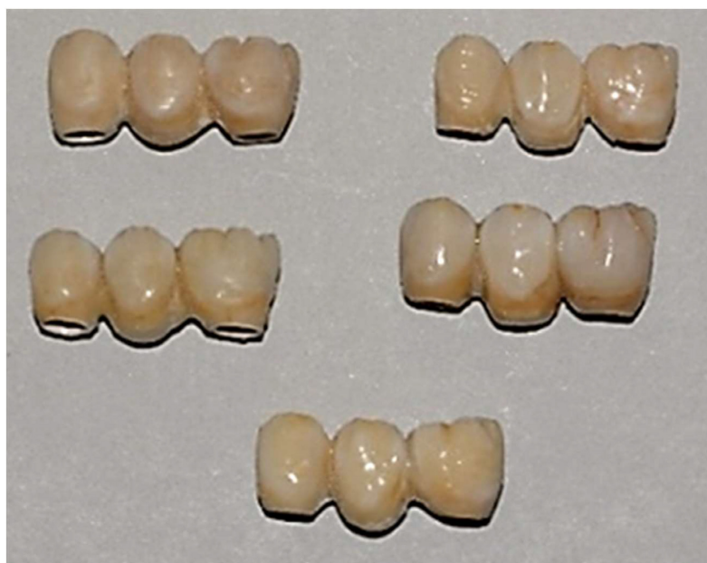
Figure 5. Samples with PEEK framework and resin composite veneering.
