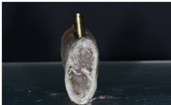
Figure 1. Two different perspectives of mandibular section simulator with two implants screwed inside: frontal view (a) and sagittal view (b).
