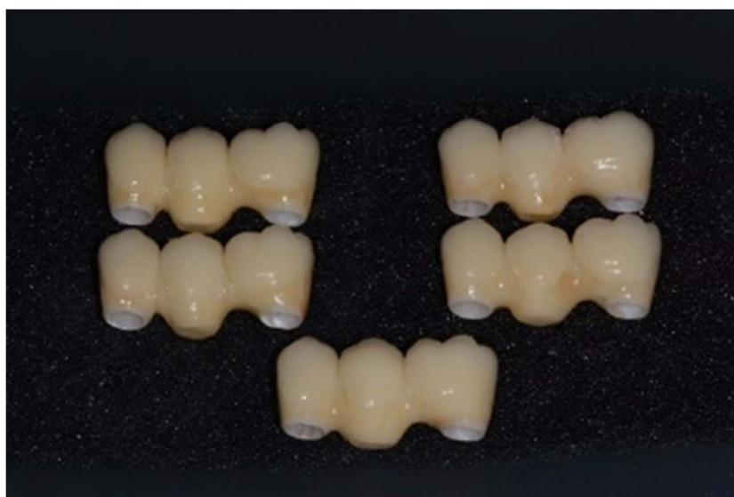
Figure 4. Samples with zirconia framework and ceramic rich in leucite veneer.
