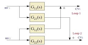
Fig. 5. Open loop diagram of a MIMO system
