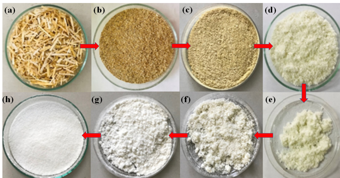
Fig. 2. (a) Raw wheat straw, (b) Grinded wheat straw, (c) Alkali treated, (d) First bleaching fibres, (e) Second bleaching fibres, (f) Final bleaching fibres, (g) Acid hydrolysis, (h) Nanocellulose
