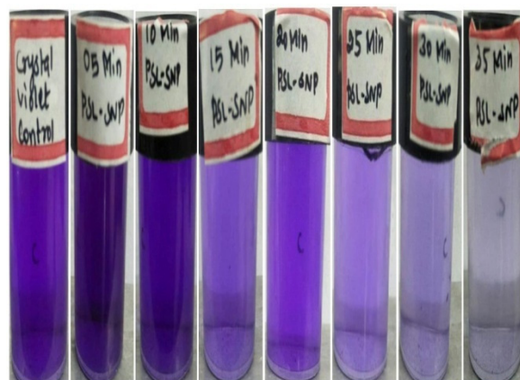
Fig. 7. Crystal violet dye degradation of Pogostemon speciosus SNPs at various time intervals
