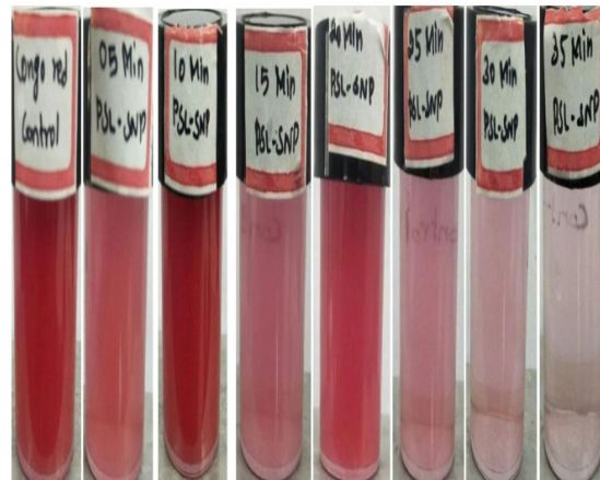
Fig.11. Congo red dye degradation of Pogostemon speciosus SNPs at various time intervals
