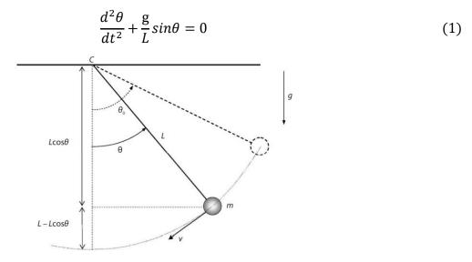
Figure 1. Scheme of a simple pendulum motion [22]
