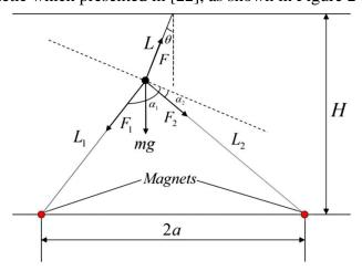
Figure 2. Pendulum system under action of double magnets [22]
