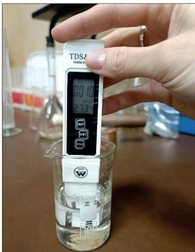
Fig. 3. Measurement of the plasticizer solution electrical conductivity using a conductivity meter
