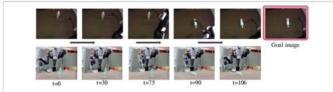
FIGURE 9 | Result of Generalization Evaluation with a PET bottle and a tree branch shown in the bottom of Figure 2. We provided a goal image showing the PET bottle toppled forward. The robot could properly detect features and generate motions to pull forward from a high position, reproducing the situation in the goal image.
