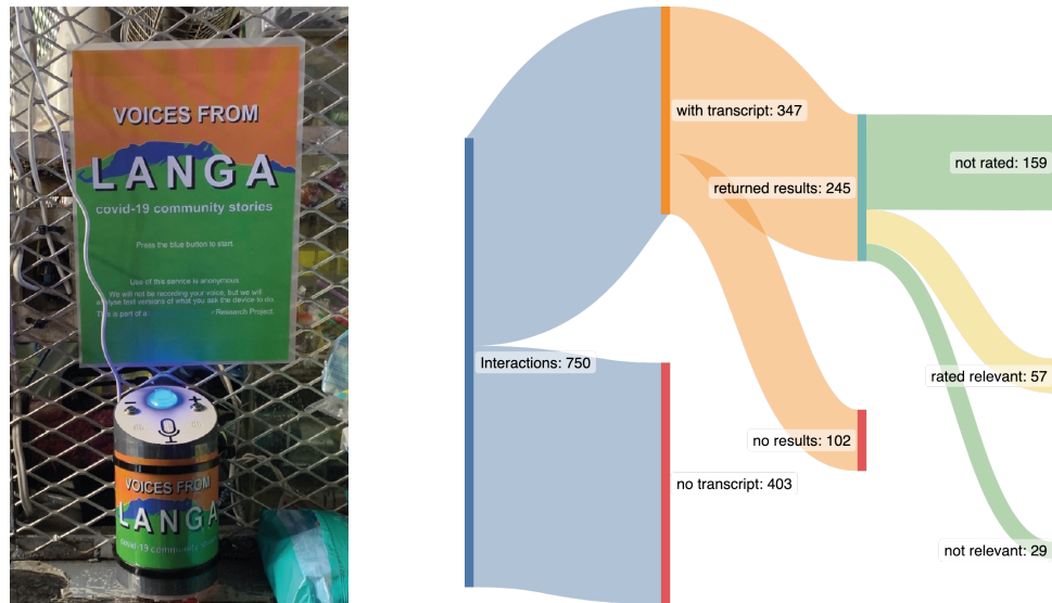
Figure 4: The ASR demonstrator as it was deployed in one of five shops in Langa over a period of three weeks (left) and a breakdown of recorded interactions on the devices (right). Around a third of queries generated a search response (i.e., an oral community story about COVID-19 that we could match to the incoming voice query). Few participants chose to respond to the post-interaction rating question, but of those who did, 66 % rated the result as relevant.
