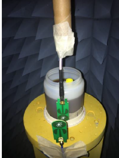
Figure 5.4: Position of the bone marrow lesion phantom inside the anechoic chamber. The phantom was placed in the centre of a rotatable table. The external PulsON P200 antenna is the transmitter, and the internal PulsON P200 antenna is the receiver.
