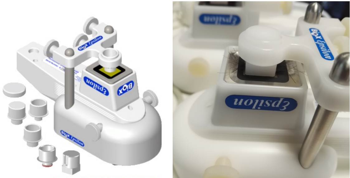
Figure 3.31. Left, the Epsilon E100 in-vitro stand as presented in the product brochure [70]. Right, the hair sample held against the sensor surface with the plastic plug during the experiment.
