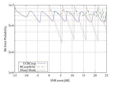
Fig. 6. ABEP for each transmission mode: red-dotted for direct mode, green-dashed for RCoopMAC, and blue-solid for UCRCoop.
