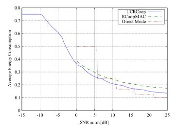
**Fig. 4.** Energy per bit  $E_b$  transmitted at the source node for each transmission mode: direct mode, RCoopMAC and UCRCoop.
