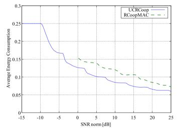
**Fig. 5.** Average energy per bit  $\bar{E}_b$  transmitted at each relay node for both cooperative strategies: RCoopMAC and UCRCoop.
