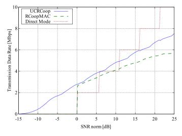
Fig. 2. Achievable data rates for different transmission modes: red-dotted for direct mode, green-dashed for RCoopMAC, and blue-solid for UCRCoop.
