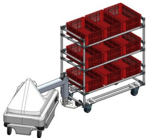
Figure 22: Towing a transport trolley with the proposed lifting and towing device attached on MiR 100
