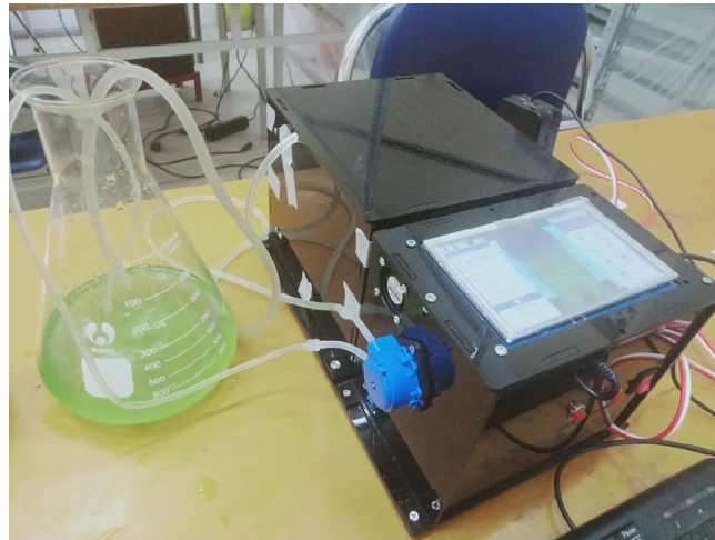
Fig. 21. The microalgal density measurement unit.
