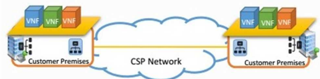
Fig 5. Decentralized VNF Deployment Model
