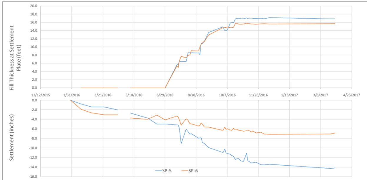
Figure 23. Fill Thickness and Settlement Plate movement with time.
