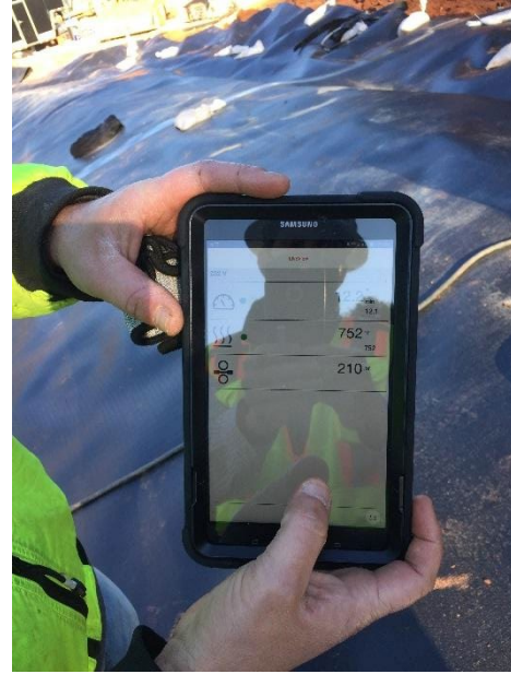
Figure 5: Tablet PC connected to the Data Acquisition Welding machine displaying seaming parameters.
