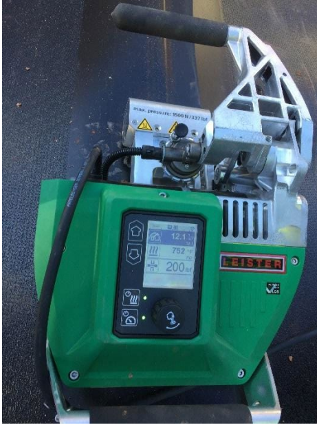
Figure 4: Data Acquisition Welding machine with visual display showing speed, temperature, and pressure.
